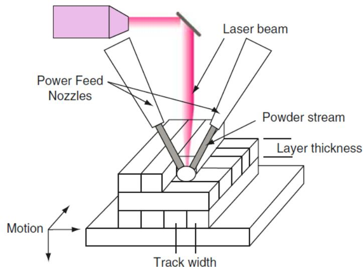
Figure 4: Directed energy deposition using a laser heat source.
