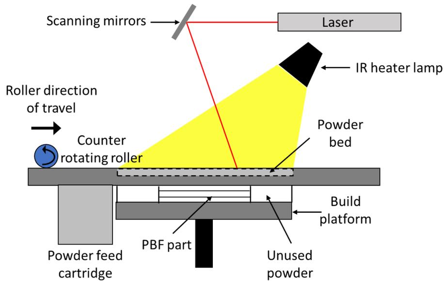
Fig. 3: Powder bed fusion process using a laser. The IR lamp can be omitted in an electron beam setup as the beam can be defocused and used to heat the powder bed.
