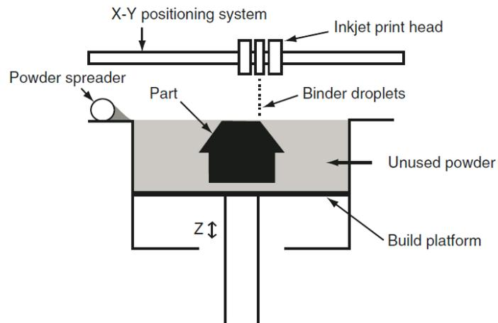
Fig. 2: Binder jetting setup. The unused powder serves as support material for the part [1].
