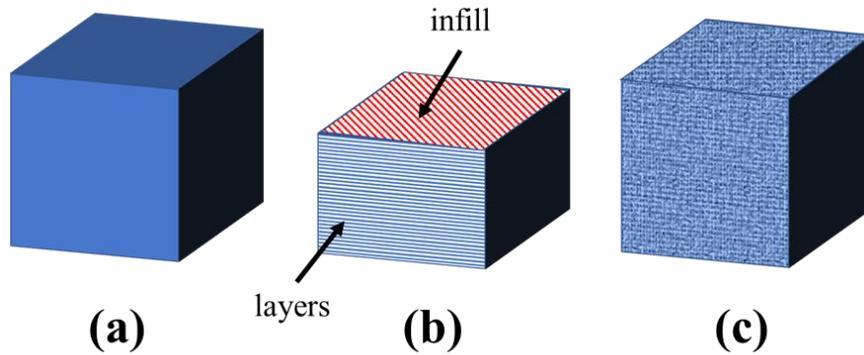
Fig. 1: AM workflow. The AM process begins with a CAD model of the part (a). Slicing software divides the part into layers and determines a toolpath to fill the inside of the part creating numerical control code (b). The numerical control code is loaded into an AM machine, and a part is produced (c).
